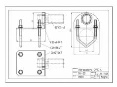
Stainless steel bracket for antenna anchoring to 25-40mm masts
