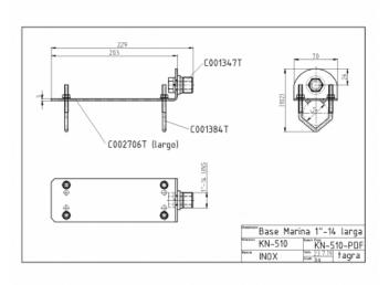
3 mm. stainless steel sheet Thread 1" -14 threads.
